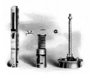
Roller Rod, Cam, Roller and Pin, Valve Crosshead, Spring and Valve with Stem
