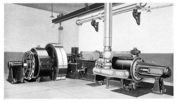
The Ames Controlled-Compression Una-Flow Engine Direct Connected with 300 K. W. Direct-Current Generator
