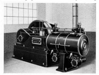
Controlled-Compression Una-Flow Engine Direct Connected with 100 K. W. Direct-Current Generator
