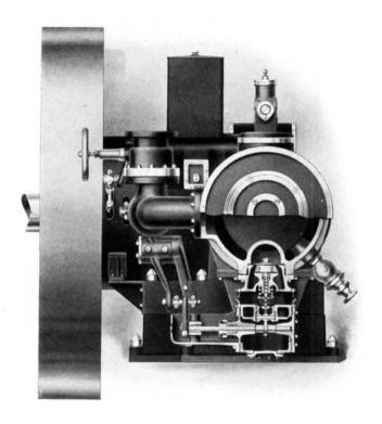
Section Through the Secondary Exhaust Bonnet and Valve
