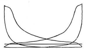
Typical Indicator Diagram From Condensing Engine
