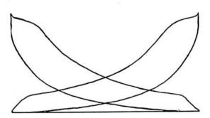
Typical Indicator Diagram From Non-Condensing Engine
