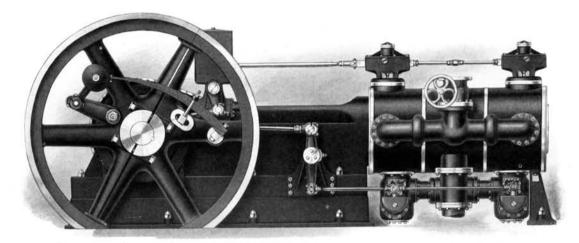
Governor and Valve Gear Side of Engine (Note Straight Line Drive Valve Gear)
