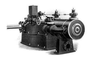
Engine Equipped with Variable Speed Valve Gear
