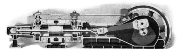
Longitudinal Section Thru Frame, Cylinder and Tail Rod Guide
